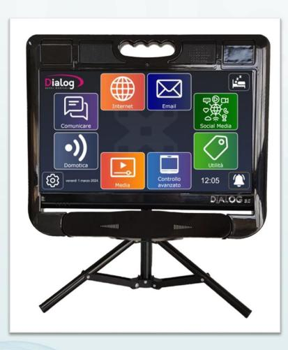
Weight: 1,5 kg Minimum Height: 45 cm Maximum Height: 60 cm Maximum Capacity: 7 kg Material: Aluminium alloy Color: Grey and black
